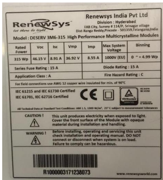
Fig. 3: rating label of test module
